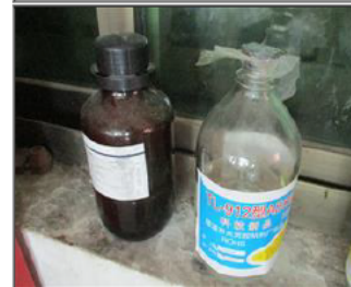
Photo of non conformity NC No valid chemical labels and secondary containment and posted MSDS.JPG
