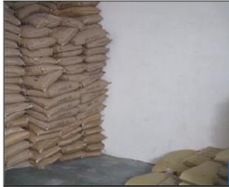
Photo of non conformity NC Raw materials were stored against the walls.JPG
