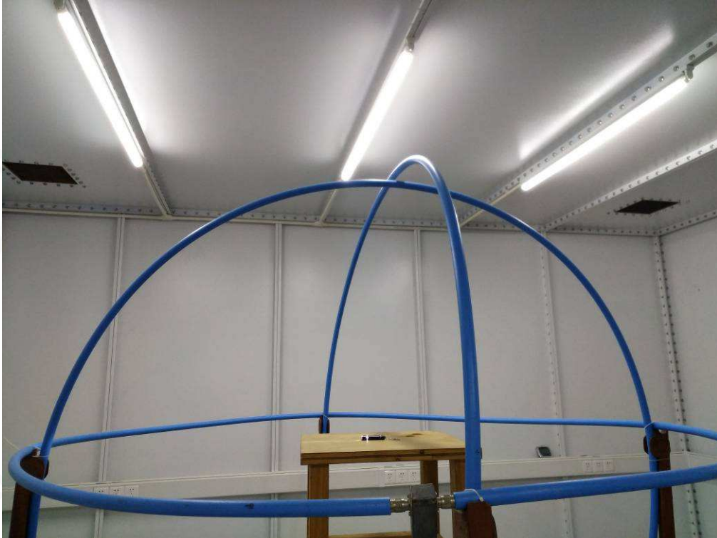
EN 61000-4-3 RS IMMUNITY TEST SETUP
