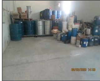
Photo of non-conformity No post the MSDS and safe label in chemicals warehouse.JPG
